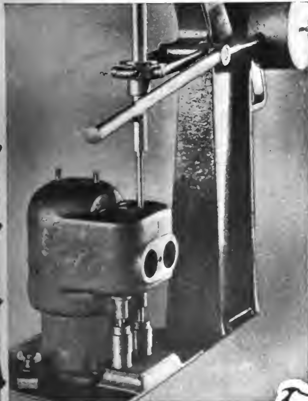
E—Valve-Grinding Machine which is Designed to Produce Reciprocating Motion, Lift, and Other Movements Made by an Expert Grinder, with the Result that Work is Done Many Times Faster and with Far Greater Uniformity Because the Machine Does not Get Tired or Careless
